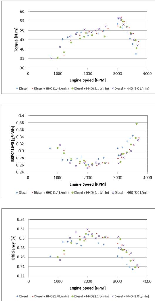
**Figure 3.** Power, torque, BSFC and efficiency as a function of engine speed (Dynamometer speed=3800)
