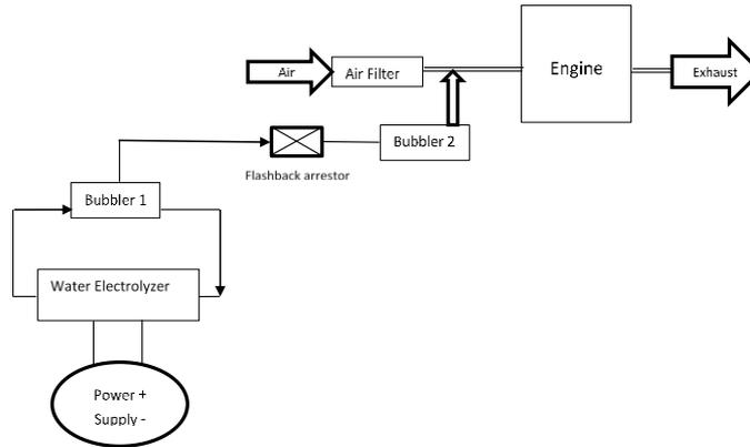
**Figure 2.** Schematic for the experimental apparatus
