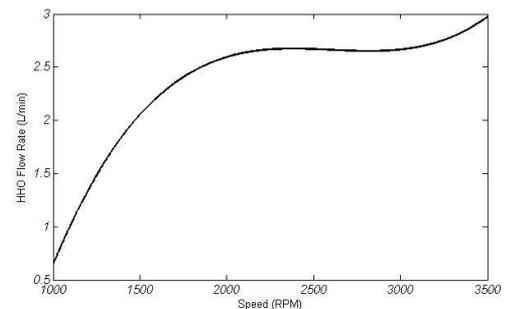
**Figure 8.** Torque based optimum HHO flow rate at each speed
