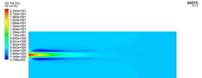
Figure 7. Oxygen concentration field for the configuration 1
