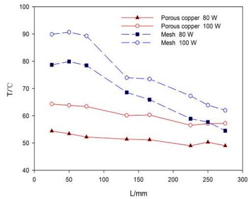
**Figure 7.** Comparison of heat pipe using porous copper foam and mesh wick
