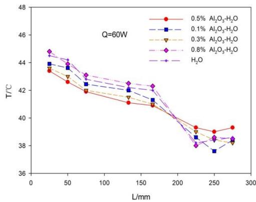
**Figure 6.** Effect of mass concentration on heat pipe heat transfer performance
