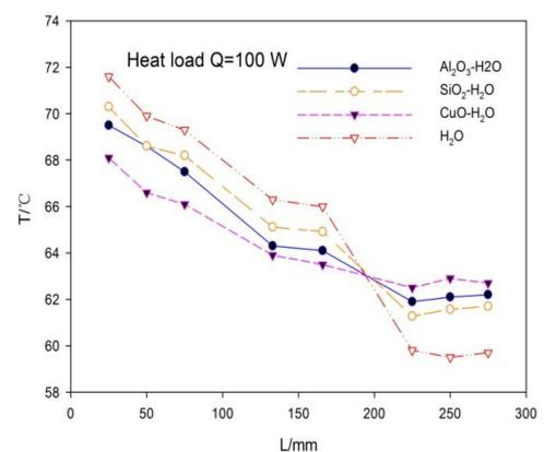
Figure 3. Temperature distribution along the heat pipes with different nanoparticles
