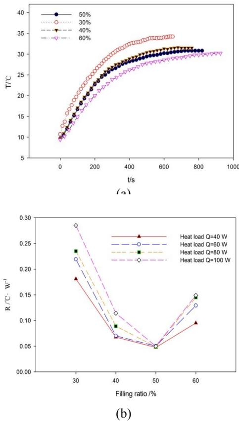
**Figure 4.** Effect of the filling ratio on the start-up and heat transfer performance, e.g., (a) change in start-up performance over time and (b) the thermal resistance with different filling ratios
