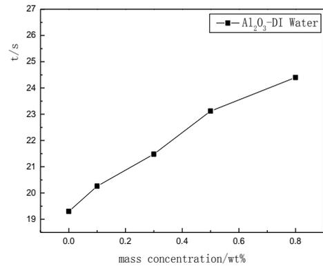
**Figure 5.** The time that the Al<sub>2</sub>O<sub>3</sub> nanofluids take to flow out with different concentrations
