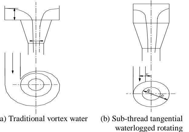
**Figure 1.** Structure schematic diagram of rotational flow generator
