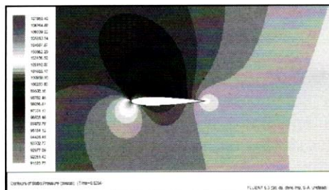
Figure 20: Iso-contour of static pressure at t = 0.8256 s.
