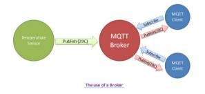
Figure 3. The use of a Broker
