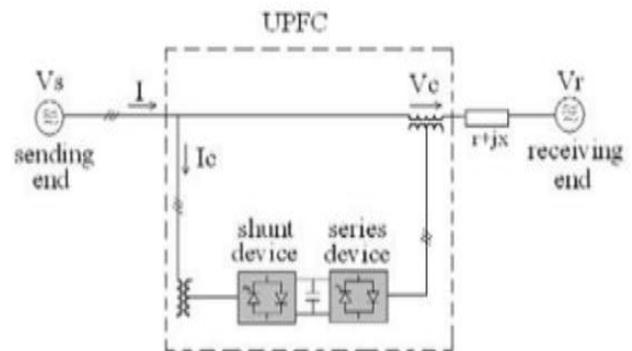
**Figure 1.** Schematic diagram of UPFC
