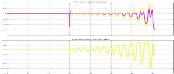
**Figure 9.** Under fault Condition power waveform
