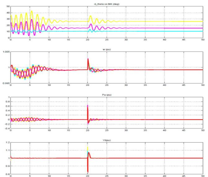
**Figure 12.** Under fault Condition machine waveform Pref. - Time [0 10], Amp [2.07 2.07], Amp [1 0] Fault- Transition Time [20 20+6/60]
