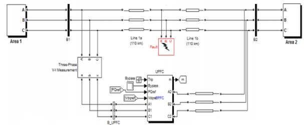
Figure 5. Simulink representation of the test model with UPFC
