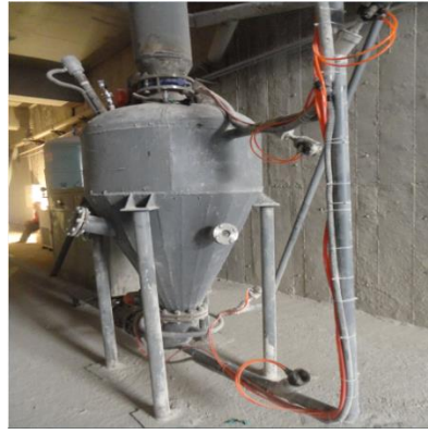
Fig2. Double-pump conveying system with constant pressure for fly ash
