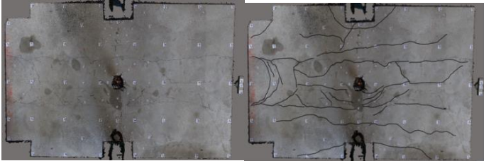
Fig.14. Distribution of Cracks on the Surface of the Box Girder after Loading
