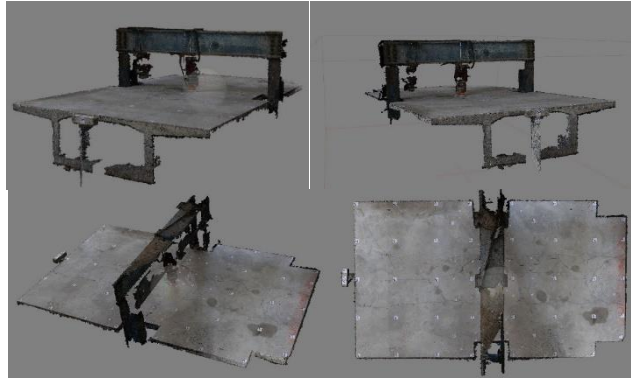
Fig.2. Three Dimensional Point Cloud Reconstruction Effect of Box Girder Specimen
