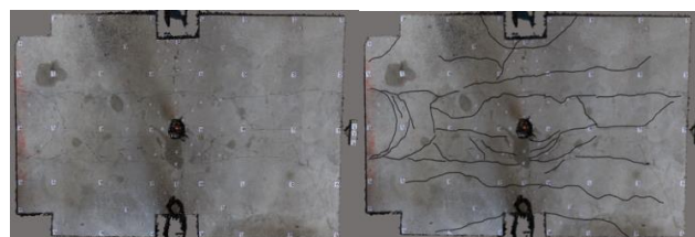
Fig.14. Distribution of Cracks on the Surface of the Box Girder after Loading
