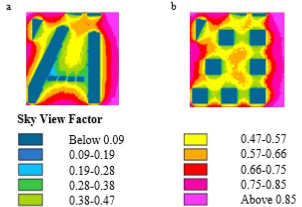
**Figure 8.** SVF - Scenarios Comparison at 13:00, h=1.5 m: a) BaseS, b) TowerS
