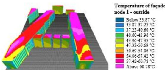
Figure 2. Temperature of facades and roofs at node 1 in ENVI-met for the Base Scenario at 13:00
