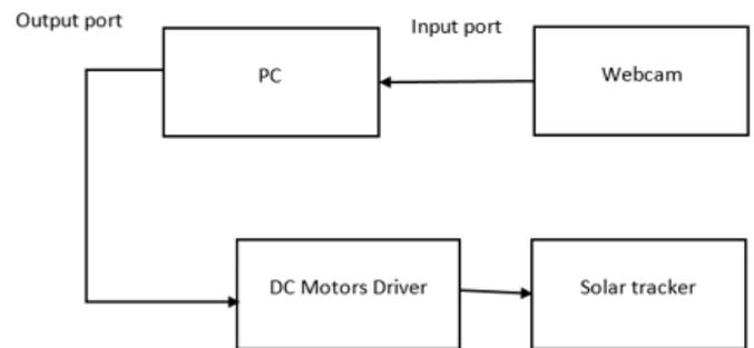
**Figure 8.** Diagram of the solar tracker system using image processing
