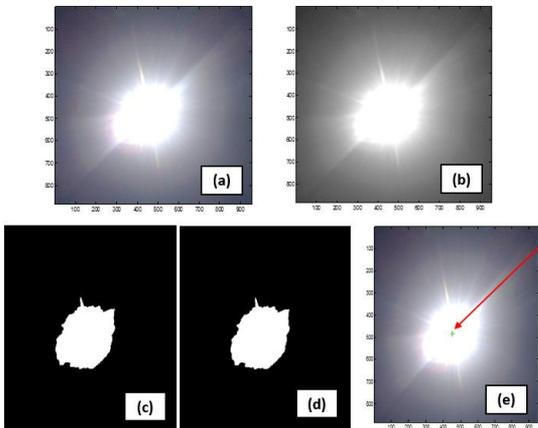
**Figure 10.** Various processing steps of the sunspot; (a) the sunspot color, (b) the sunspot grayscale, (c) binarization of the sunspot, (d) expansion of the morphology of the sunspot, (e) center detection of the sunspot (px=453.9255, py=483.6863)
