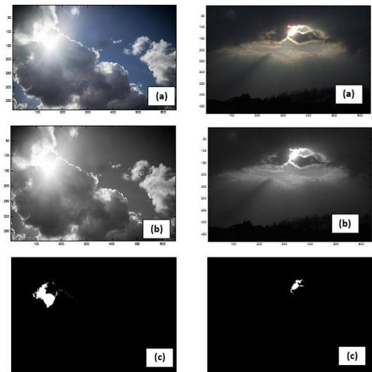
**Figure 11.** Various processing steps of the sunspot with the percentage of the circular shape of the sun less than 75%; (a) the sunspot color, (b) the sunspot grayscale, (c) the binarization of the sunspot
