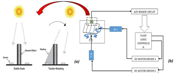
**Figure 3.** (a). Light sensor array design. (b). Block diagram for the sun tracker system [33]
