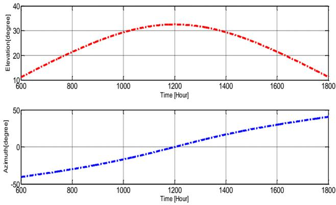
**Figure 12.** Heliostat's movements (azimuth and elevation) - day 50 with cloud between 06:00 and 18:00
