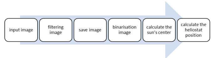
**Figure 7.** Image processing algorithm
