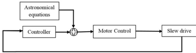
**Figure 1.** Operational principles of open-loop solar tracking control
