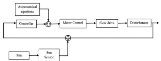
**Figure 4.** Operational principles of hybrid (open-loop/closed-loop) motion control
