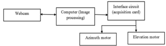
**Figure 6.** Experimental assembly block diagram for image processing technique
