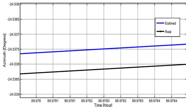
**Figure 14.** Heliostat real trajectories and estimated by the ANN (azimuth) - day 50
