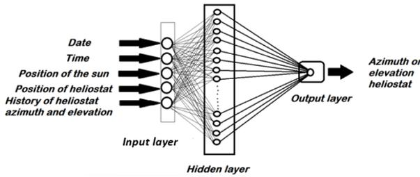
**Figure 9.** Neural Network movement estimating model
