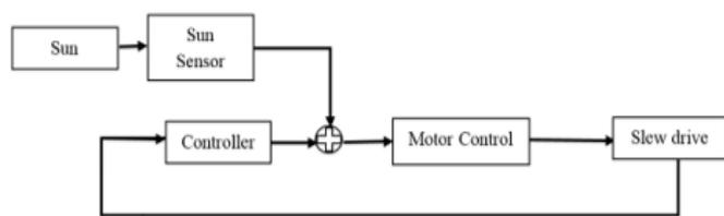
**Figure 2.** Operational principles of closed-loop solar tracking control
