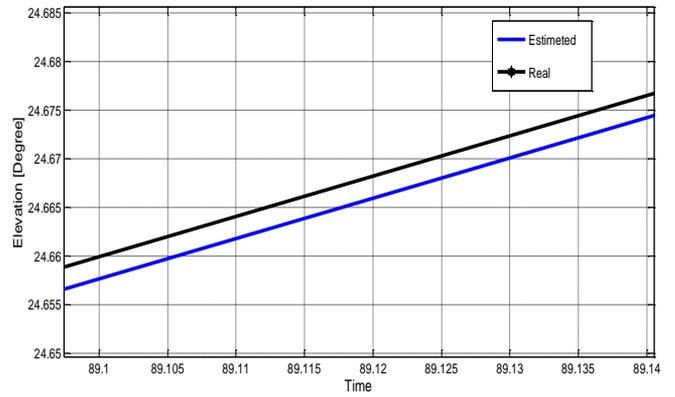
**Figure 16.** Heliostats real trajectories and estimated by the ANN (elevation) - day 50
