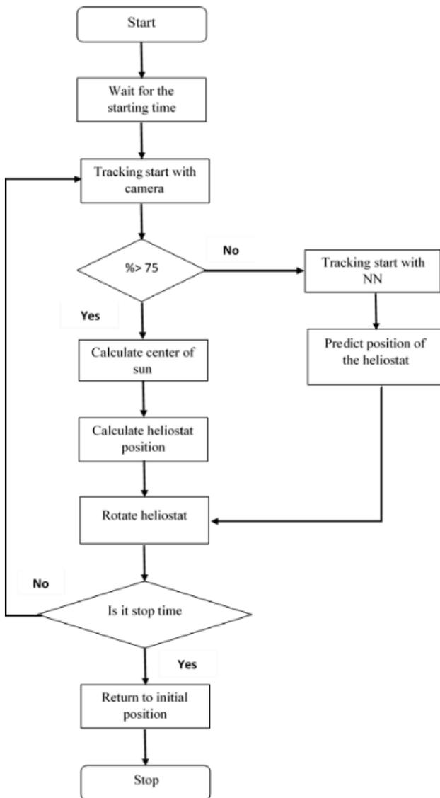
**Figure 5.** Flowchart of the hybrid algorithm of heliostat control
