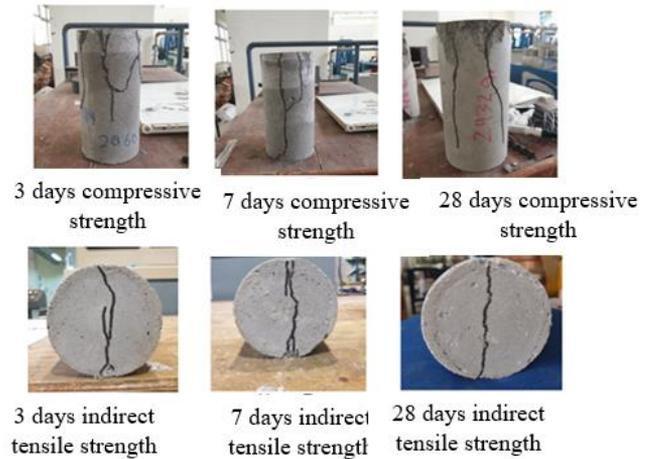
Figure 9. Mixed III crack pattern of lightweight concrete
