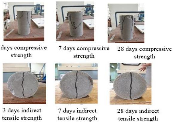
Figure 8. Mixed II crack pattern of lightweight concrete
