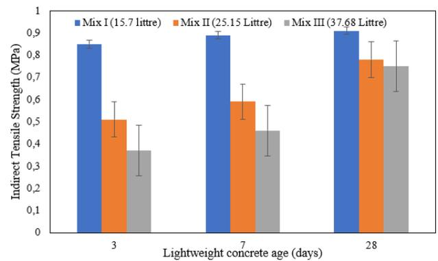
Figure 6. Comparison diagram between curing age and indirect tensile strength
