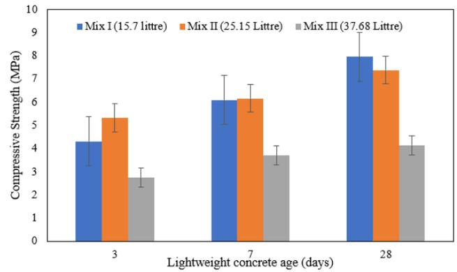
Figure 5. Comparison diagram between curing age and compressive strength
