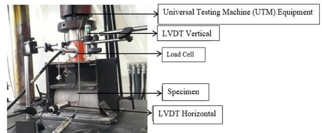
Figure 3. Indirect tensile strength test
