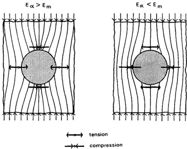
**Figure 4.** When two-phase composites with a spherical inclusion contained in a matrix are subjected to compressive loadings, a general model of the stress distribution is used.  $E_{\alpha}$  is the inclusion's elasticity modulus, while  $E_m$  is the matrix's elasticity modulus
