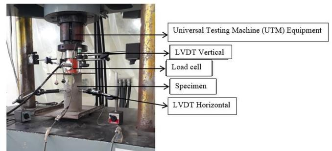
Figure 2. Compressive strength test
