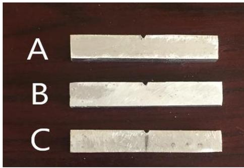
**Figure 3.** (a) Schematic diagram of sample for impact test, (b) Samples before fracture
