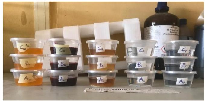
**Figure 4.** Corrosive media containing AZ31Mg-CaCO<sub>3</sub> samples: Plasma, Blood, Urine, NaCl and H<sub>2</sub>O
