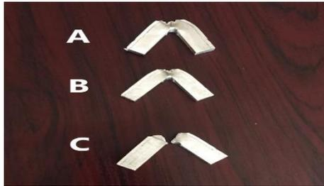
Figure 8. Impact samples after fracture
