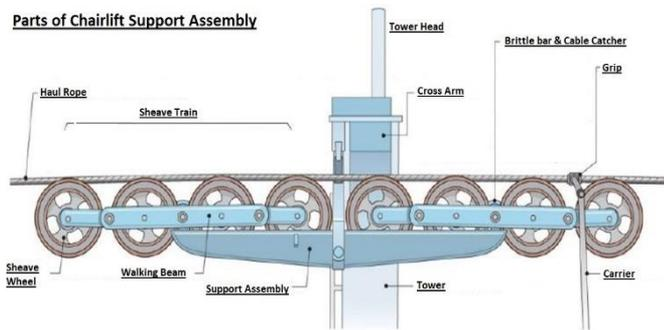
Figure 3. Gondola pillar support mechanism [23]
