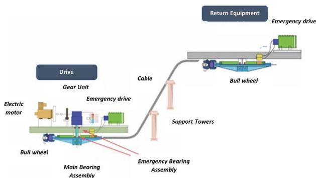
Figure 1. Schematics for Gondola cable car system [12]
