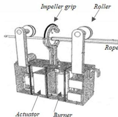
Figure 5. Powered impeller deicing device [42]
