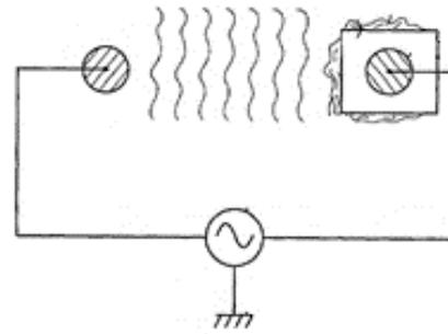
Figure 4. High frequency de-icing circuit schematics [55]
