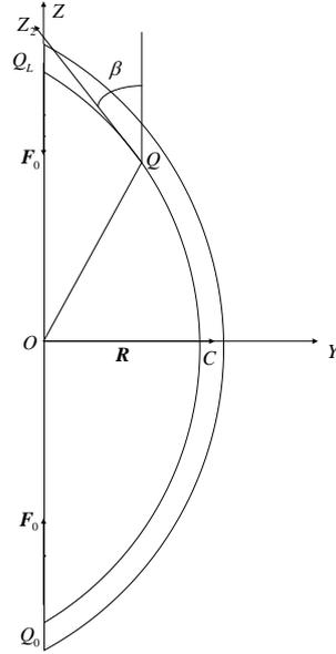
Figure 2. Establishment of coordinate system of cable under plane constraint
