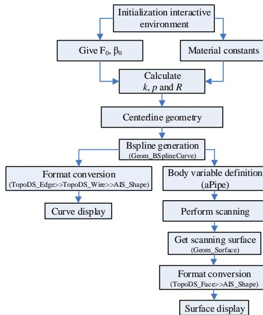
Figure 4. Development flow chart of cable module under plane constraint
