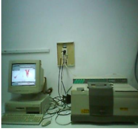
Figure 1. Experimental setup for transmittance measurements
