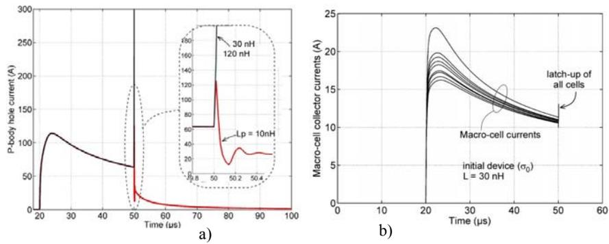
Figure 9. a) P-body hole current ( $L_p=10\text{nH}$ , 30, and 120nH); b) Distributed currents for short circuit operation for  $L_p=30\text{nH}$  and “initial” device (latch-up)
