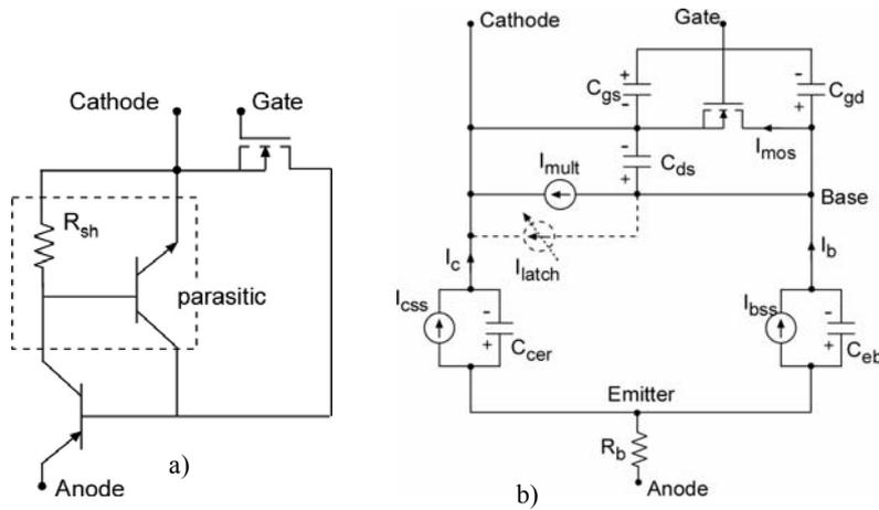
Figure 3. a) Parasitic npn transistor; b) Electrical model used for each IGBT macro-cell
