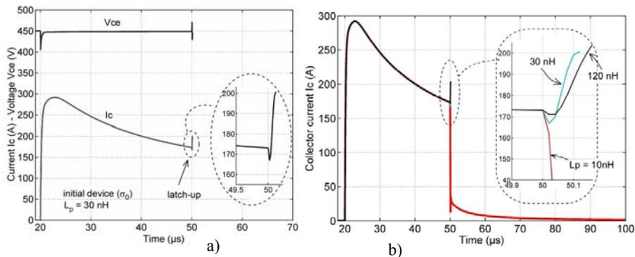
Figure 8. a)  $L_p = 30$ nH and “initial” device (latch-up); b) Collector current ( $I_c$ ) for different values of parasitic inductance ( $L_p = 10$  nH, 30 nH to 120 nH)
