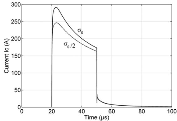
Figure 5. Top-metal ageing effect on the short-circuit current
