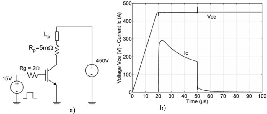
Figure 4. a) Electrical circuit; b) Simulated short-circuit operation ( $L_p=10nH$ )
