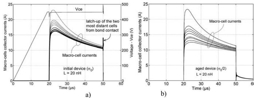
Figure 10. a) Distributed currents for short circuit operation for  $L_p=30\text{nH}$  and “initial” device (latch-up); b) Short circuit operation for  $L_p=20\text{nH}$  and “aged” device (no latch-up)
