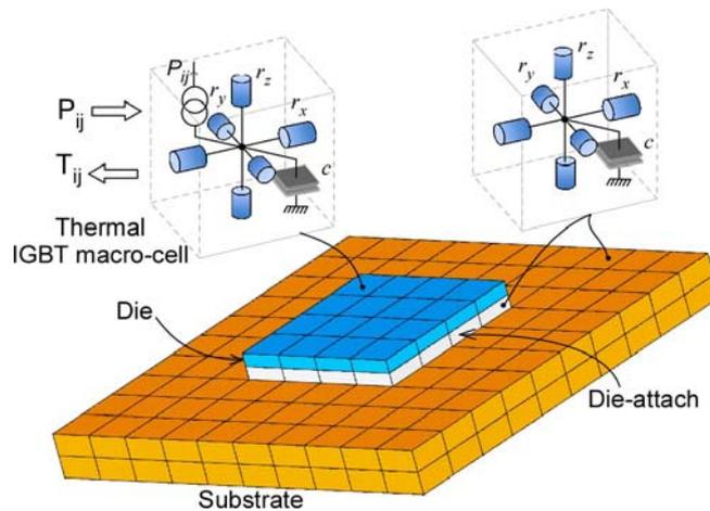
Figure 1. Thermal component
