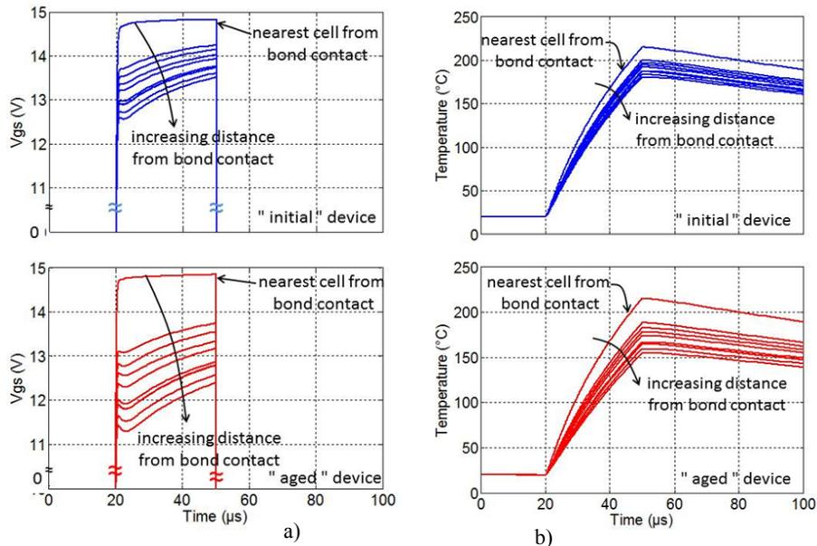
Figure 7. a) Macro-cell inner gate-to-source voltage distribution; b) Macro-cell temperature distribution
