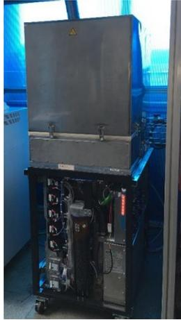
Figure 3. SOFC generator
