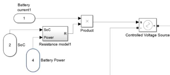
Figure 9. MATLAB modifications to lithium model
