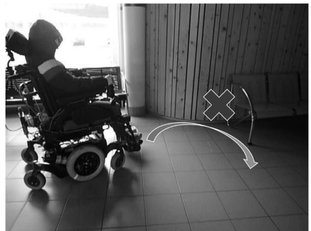
Figure 3. Wall detection and trajectory restoration
