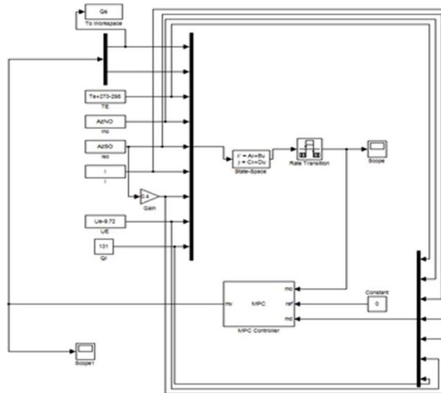
Figure 5. MPC Simulink model
