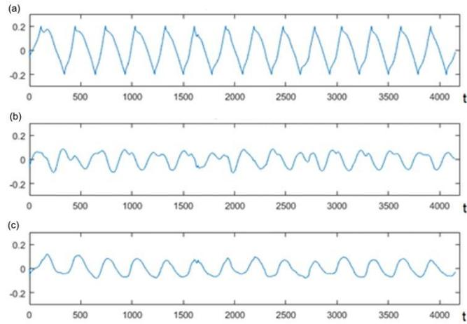
Figure 7. PMV index with three different controller types: (a) ON/OFF; (b) PID; (c) MPC
