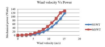
Figure 9. Graph shows the mechanical power vs wind velocity
