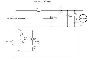
Figure 2. DC to DC power converter
