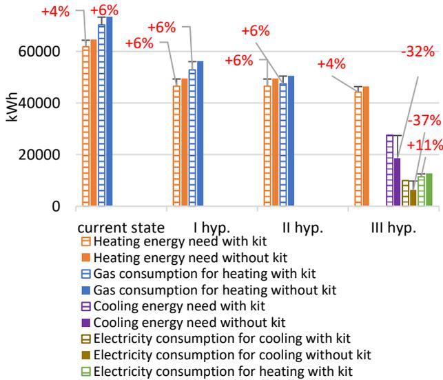
Figure 9. Energy need and consumption, with and without the kit [kWh]
