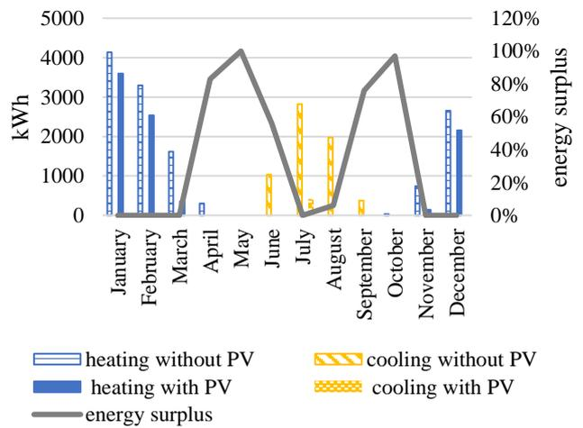
Figure 12. Third refurbishment hypothesis: electricity consumption for heating and cooling with and without PV modules
