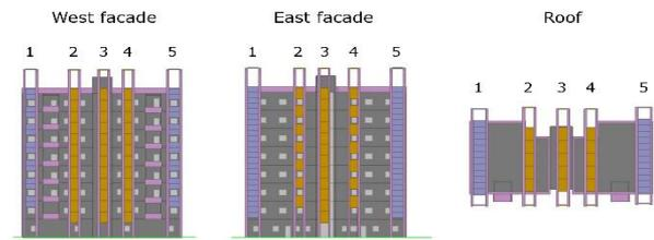
**Figure 8.** Arrangement of the five kits (PV modules in blue, thermal solar modules in orange)
