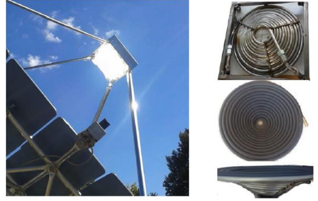
Figure 3. Receiver and absorber of TGS H2.0 (Project S.r.l.)
