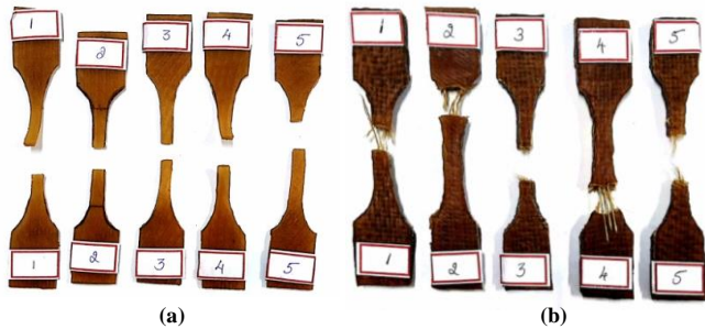
Figure 7. Specimen of (a) rubber and (b) jute-rubber after experimental tensile test
