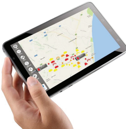
Figure 4: 2D map visualisation of a sample flood-prone area within the Basento basin. The billboards of the structures and infrastructures display different colours according to the level of criticality simulated by hydraulic models.
