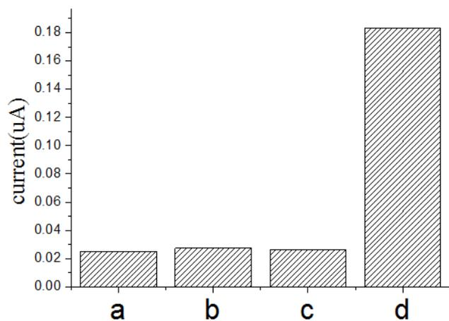
Figure 4. Comparison of the signal of dsDNA modified electrode when incubated in prepared solution contain  $10^{-6}$  mol/L PdS nanoparticle-labeled DNA probe with (a) without thrombin, (b) with  $3.0 \times 10^{-7}$  M of lysozyme, (c) with  $2.5 \times 10^{-8}$  M of BSA, (d) with  $2.15 \times 10^{-10}$  M of thrombin.
