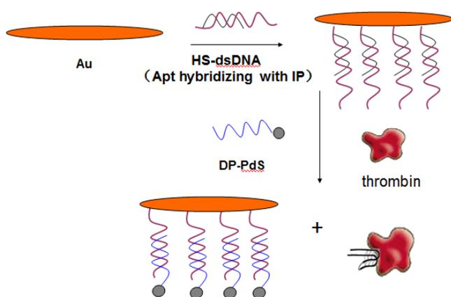
Figure 1. Schematic representation of the procedure to prepare electrochemical biosensor for the determine of thrombin via target protein-induced strand displacement and hybridization.
