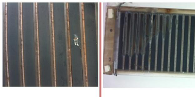
Figure 10. Cracking in the surface cells of the IP-SOFC.
