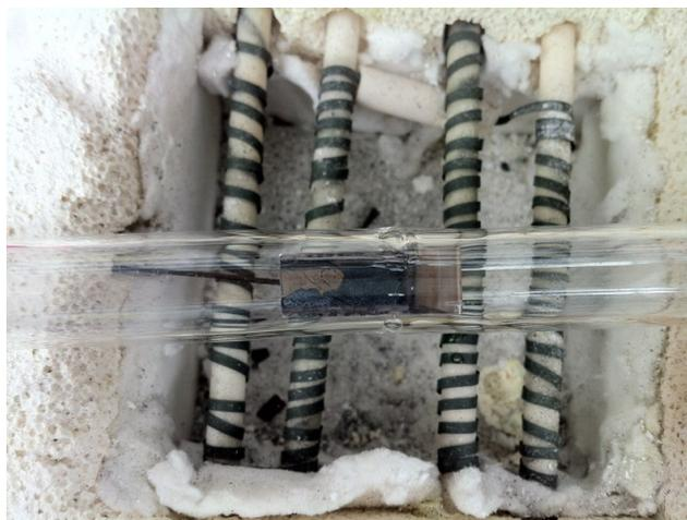
Figure 2. The IP-SOFC piece inside a quartz tube in furnace.
