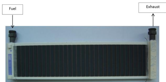
Figure 1. Integrated Planar Solid Oxide Fuel Cell (IP-SOFC).
