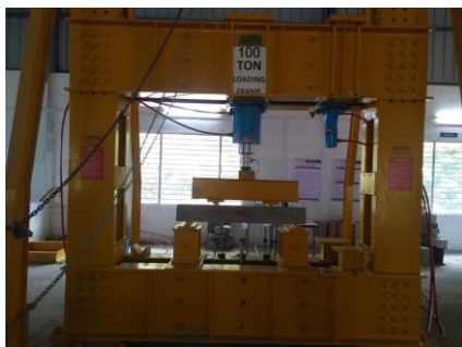
Figure 2. Flexural strength test of concrete specimen
