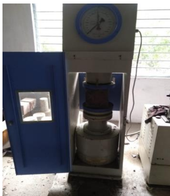
Figure 1. Compressive strength test of concrete specimen
