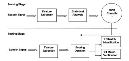
Figure 7. Two different phases of the speaker recognition system
