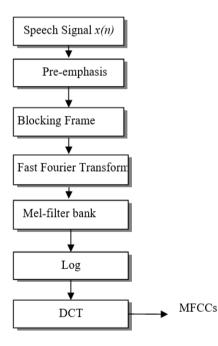
Figure 8. Block diagram of MFCCs
