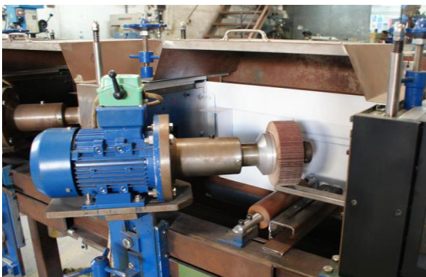
Figure 7. AC motor with flap wheel
