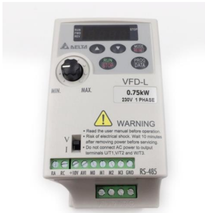
Figure 9. Variable frequency drive (VFD)
