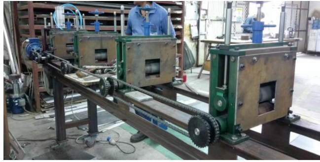
Figure 21. Roller guide mounted on base frame
