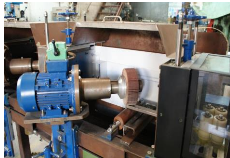
Figure 17. Sliding polishing head guard
