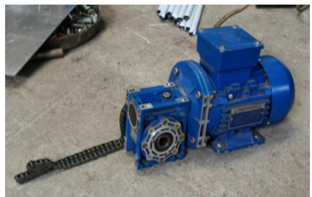
Figure 8. Worm gearbox motor
