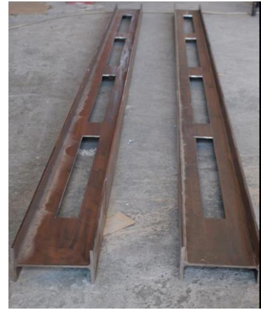
Figure 3. Mild steel I- Beams
