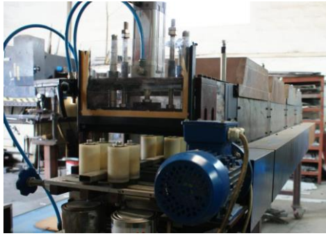
Figure 13. Nylon guide rollers
