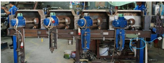
Figure 23. Final assembly of the polishing machine
