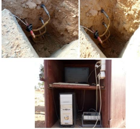
Figure 7. Soil temperature Probes (S1, S2, S3, S4, S5, S6), implanted every “0.20 m”
