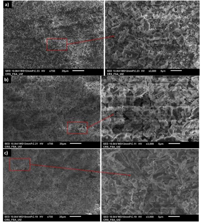
**Figure 10.** SEM images of the composites a)-OP0, b)-OP8, c)-OP16
