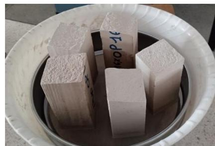
Figure 9. Water absorption by capillarity
