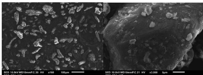
**Figure 3.** Microstructure of olive pomace powder
