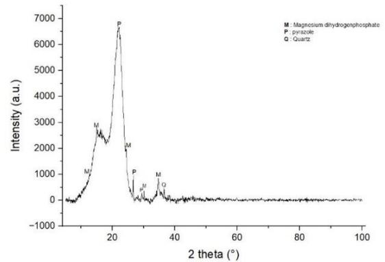
**Figure 5.** Diffractogram of olive pomace waste
