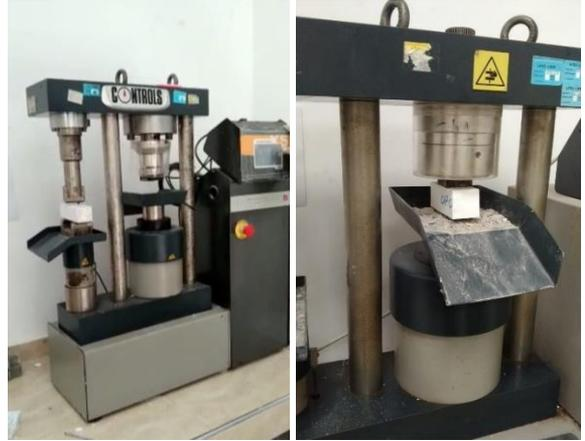
Figure 8. Compression and flexural test
