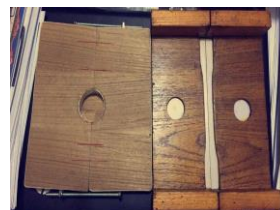
Figure 6. Molds for tensile and compressive testing samples (Made of Wood)
