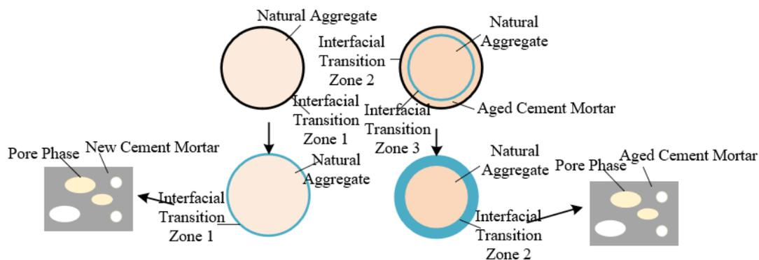
**Figure 2.** Evolution process of the interfacial transition zone
