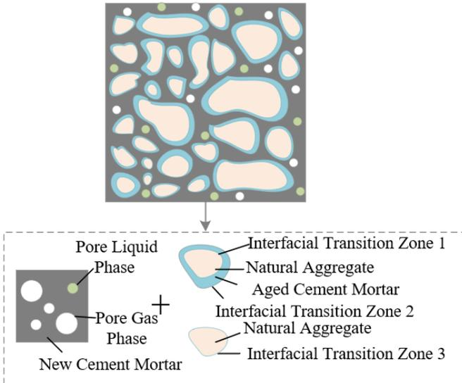
**Figure 3.** Principle of multiphase heat conduction analysis in building solid waste recycled concrete
