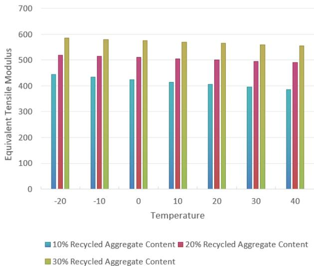
**Figure 7.** Equivalent tensile modulus and temperature relationship of building solid waste recycled concrete
