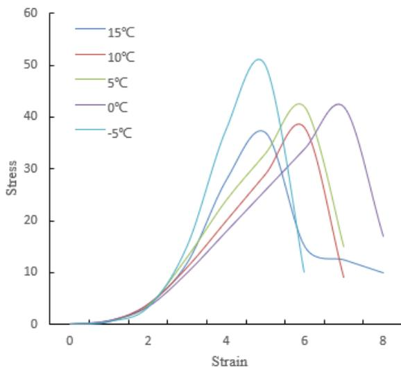
**Figure 6.** Stress-strain curve of building solid waste recycled concrete
