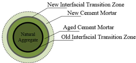
**Figure 1.** Structure of building solid waste recycled concrete
