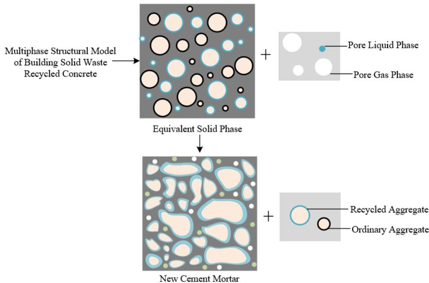
**Figure 4.** Theoretical model of thermal conductivity coefficient for building solid waste recycled concrete
