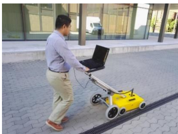
Figure 14. 300MHz GPR was used to detect the urban roads
