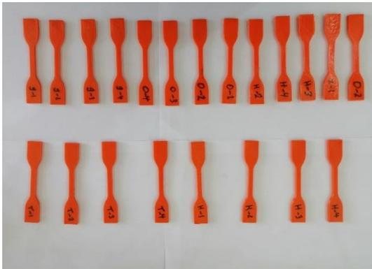
Figure 3. The 3D-printed tensile specimens
