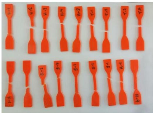
Figure 4. The fractured 3D-printed tensile specimens
