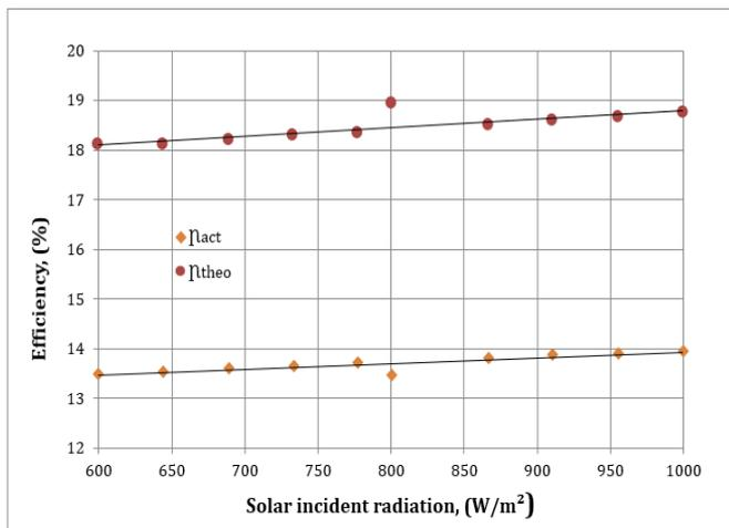
**Figure 5.** Actual and theoretical efficiencies against the incident solar radiation for YHM-205-27P solar module
