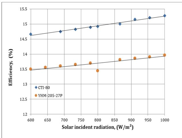
**Figure 8.** Actual efficiency for both CTI-80 and YHM-205-27P
