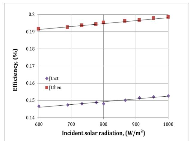
**Figure 6.** Efficiencies verses the power incident for CTI-80 solar module
