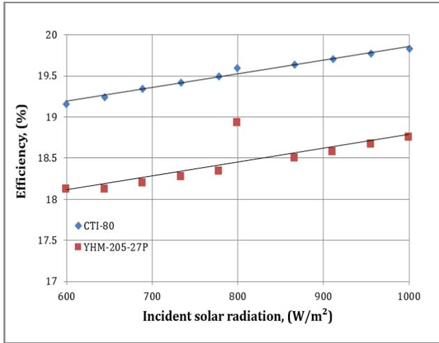
**Figure 7.** Theoretical efficiency for both CTI-80 and YHM-205-27P
