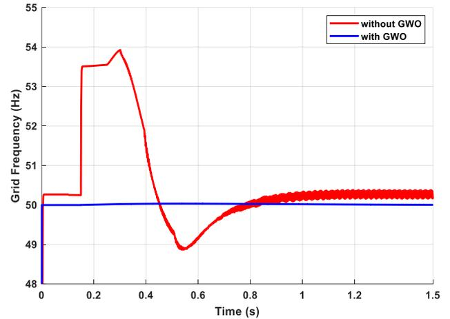
**Figure 3.** The frequency response of two systems under test. without optimization (dashed), with GWO (solid)
