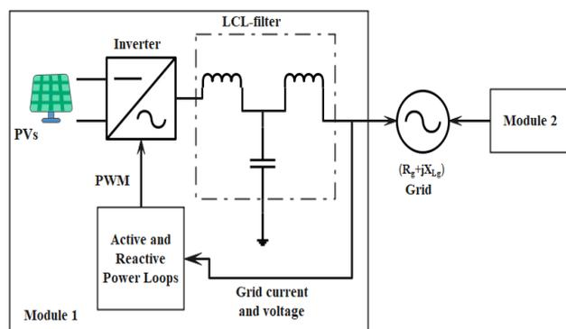
**Figure 1.** A power system grid with two VSGs in parallel (module 1 and module 2)
