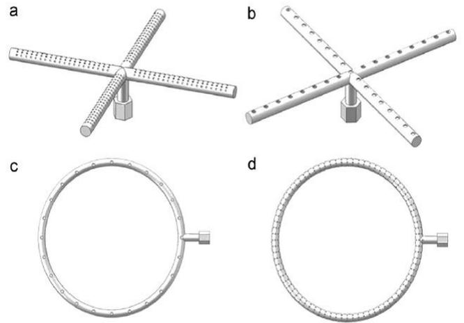
**Figure 6.** Photos of the air injection nozzles: (a) NozzleNo.1, cross, 384holes; (b) NozzleNo.2, cross, 24holes; (c) NozzleNo.3, circular, 24holes; (d) Nozzle No.4, circular, 384 holes
