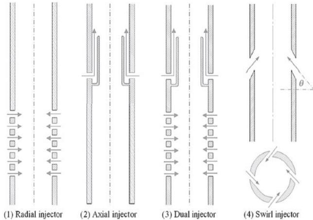
Figure 7. Schematic of air injectors design
