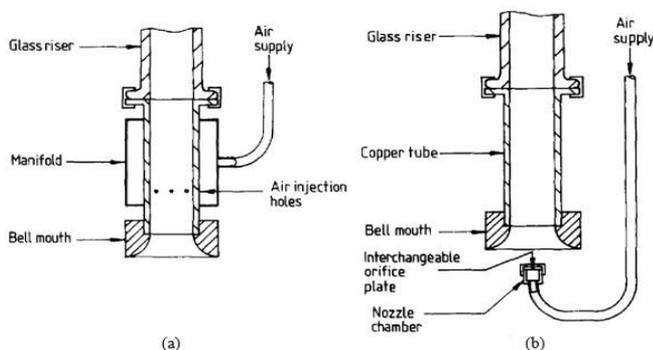
**Figure 3.** Details of the foot piece designs tested: (a) the air-jacket injector, (b) the nozzle injector
