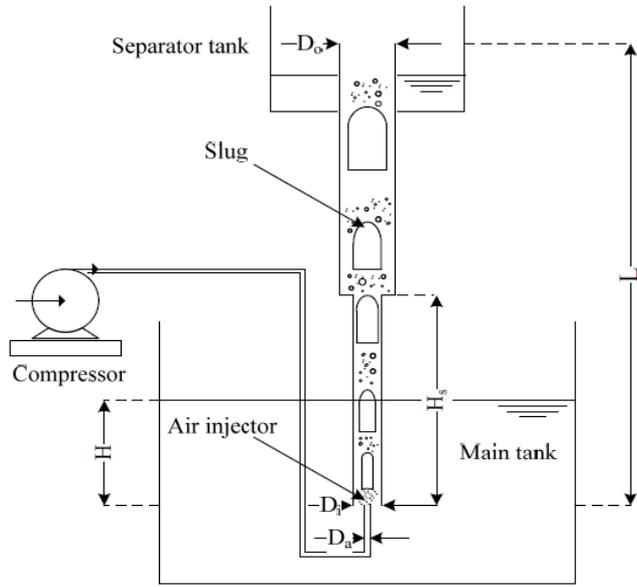
**Figure 5.** Schematic of airlift pump with step geometry
