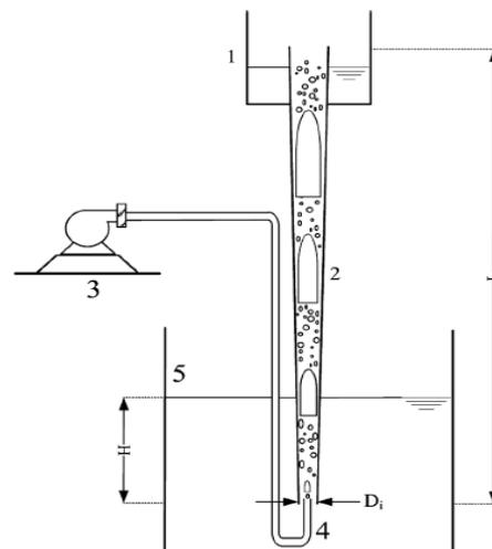
**Figure 4.** Schematic of airlift pump
